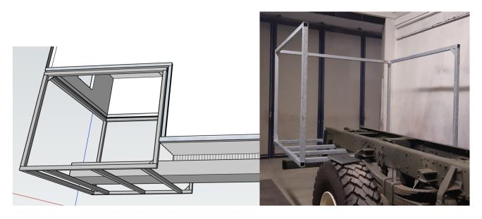
The entire garage structure is not linked to the living cell, but the two parts can swing independently.
